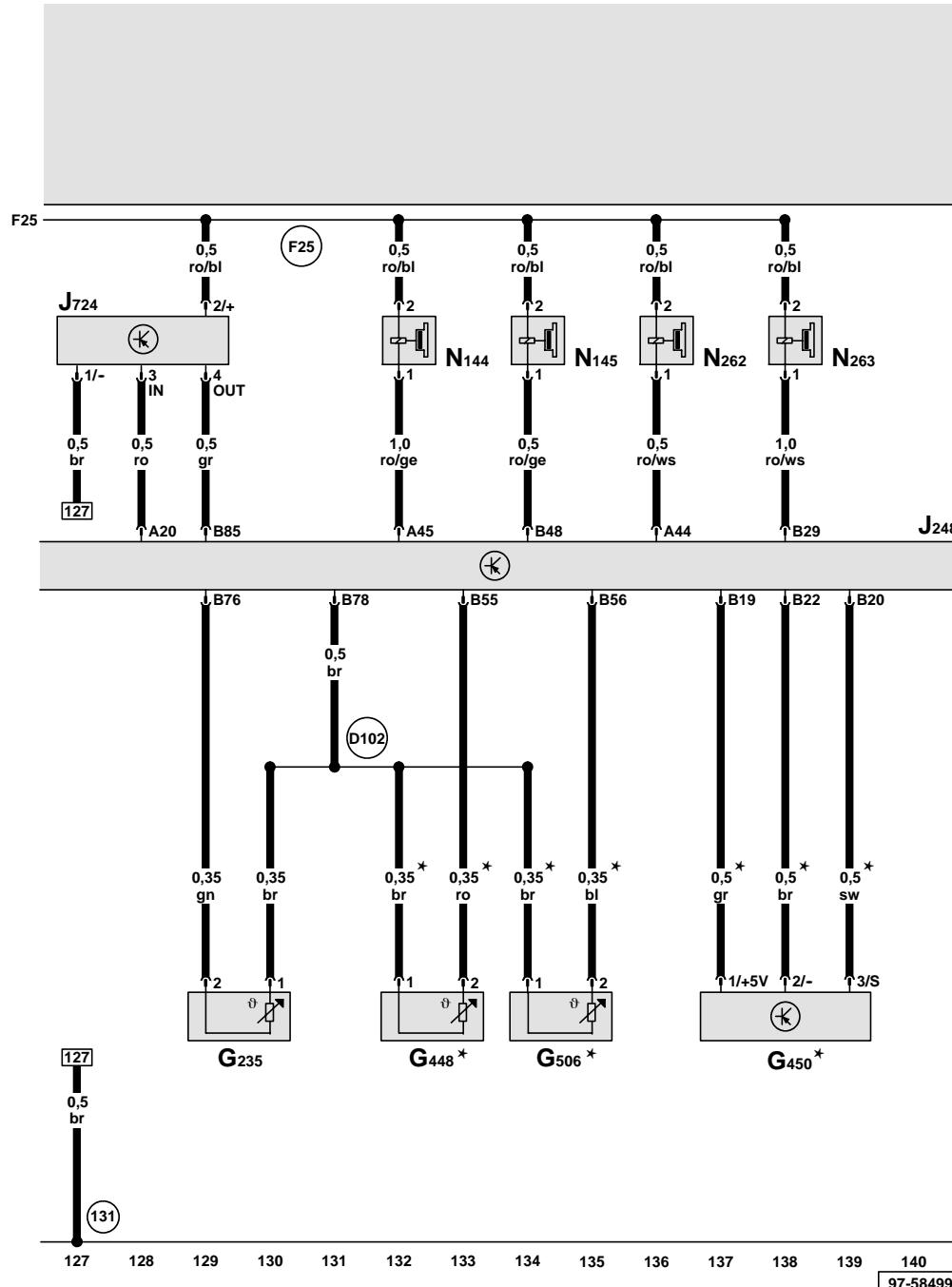
Diesel direct injection system control unit, turbocharger 1 control unit, exhaust gas temperature sender, electro-hydraulic engine mounting solenoid valve, gearbox mounting valve, temperature sender before particulate filter, exhaust gas pressure sensor 1
